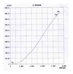
Note: parameters of pressure test with rubber gasket
