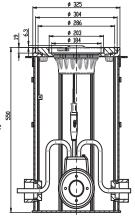
Embedded installation on the 12" deep base with the 12/8 inches adapter ring
